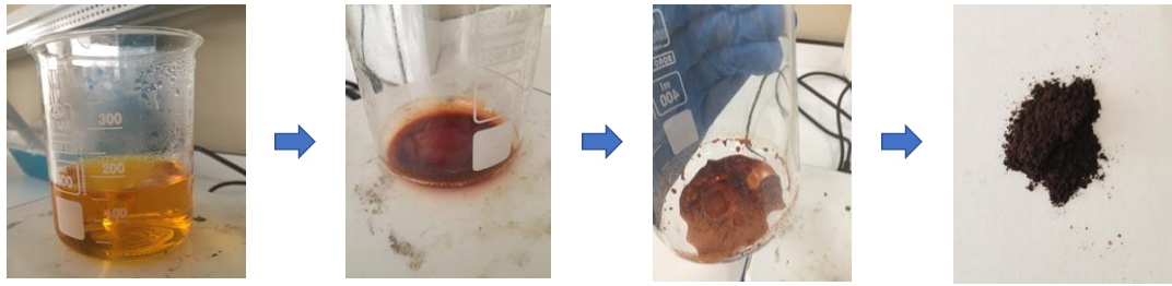
Figure 3.1: Synthesis steps of barium hexaferrite
